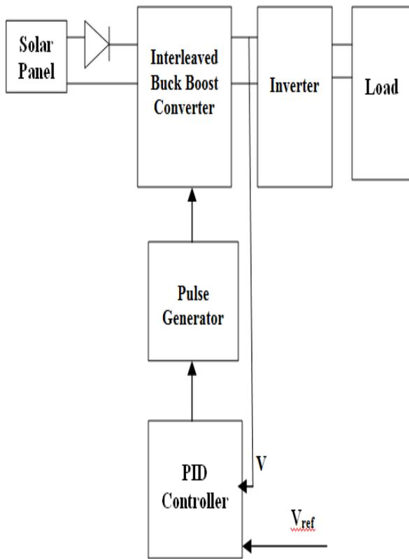
Fig. 1. Proportional Integral Derivative Controller in Photovoltaic interleaved buck boost converter for solar system system
