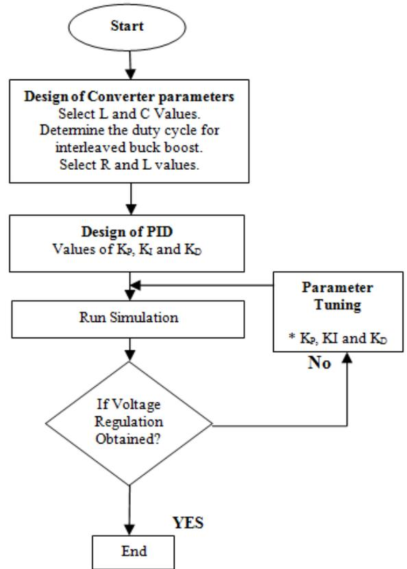
Fig. 2. Flow Chart for Design of Proportional Integral Derivative Controller
