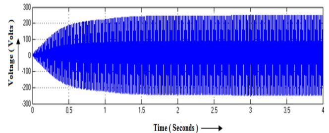
Fig. 6. Output voltage of inverter with PID controller
